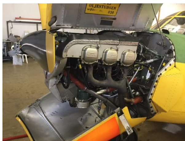
Den 6-cylindriga motorn Lycoming O-435
